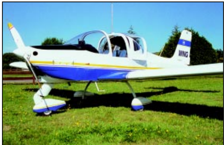
Rearward sliding canopy allows for simplified entry and exit. Pilot and passenger enter over the wing leading edge.
